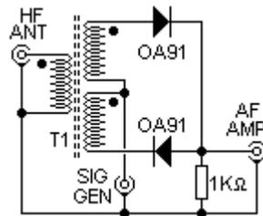
T1 is a Triflar wound component on a 1/2" ferrite ring. Twist together 3 lengths of thin enamelled wire and wind 17 turns on the ferrite ring. One winding is for the antenna and the other two are for the mixer. The black blobs by the T1 windings indicate the polarity of the transformer. All of the black blobs are the same end.
