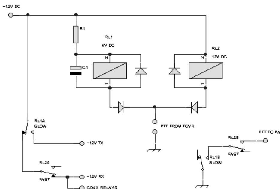
The way you interlink the "fast" and "slow" contacts on the two relays depends on your switching requirements. The sequence must be:
